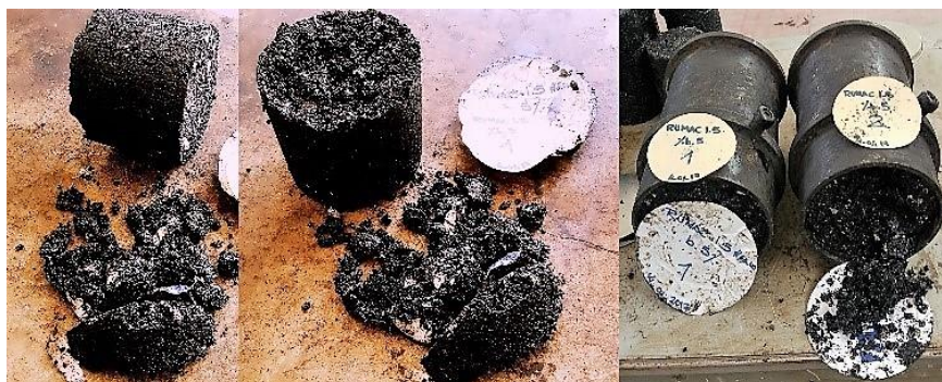
Fig. 1 Swelling effect on rubber-modified HMA samples of \varnothing 150 \times 120 \text{mm} manufactured according to SGC
