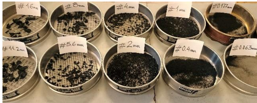
Fig.8 Sieve analysis of the rubber from discarded truck-tires
